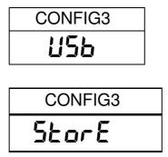
Press [Setup/Enter] to confirm the action. Or press [ $\rightarrow 0/T \leftarrow / Esc$ ] to escape back to the original USB display.
