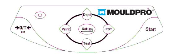
The keypad has second function keys to allow a selected menu item or value to be incremented or changed. Right/left shift to change the active digit and up/down to increment or decrement a value.
